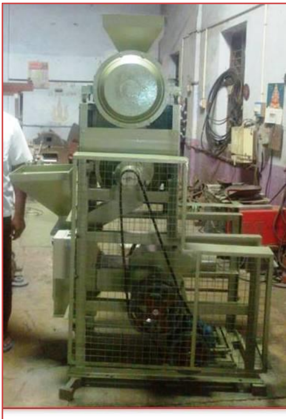
Double Chamber Centrifugal Dehuller- TNAU
