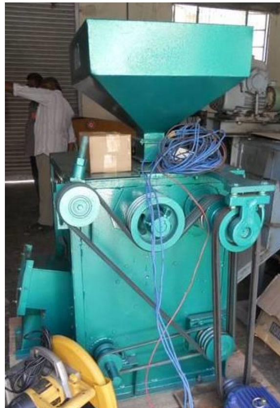
Rubber Roller Dehuller- CFTRI
